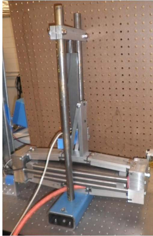
Figure 17 Complete Terfenol-D powered bulk motion assembly
