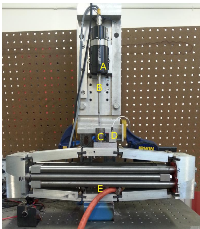
Figure 33 Experimental setup, comprised of CU-18 vibration transducer (A), titanium horn (B), lower die (C), displacement sensor (D), bulk motion transducer (E)
